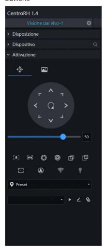
With the controls at the bottom of the panel, you can also set and recall presets and tours.
