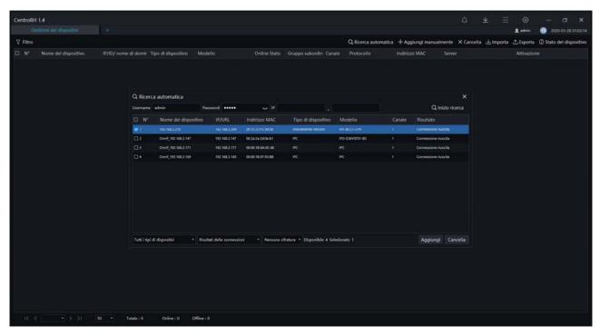
To add a camera to the program you have to select it and press ADD. Remember, you can manage CentroRH just our RH Series cameras. It does not work with other cameras.
