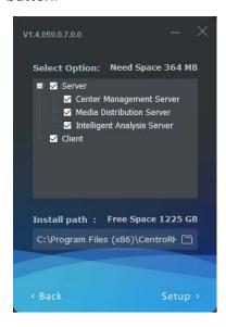
In this window you can also choose to install the program in a client version for display only. If you install the software components in different PC you will need to configure each component in the IP of the PC that contains the Center Management Server using the Server Manager tool, which troveri installed to the utility of the program and whose icon is in the taskbar.
